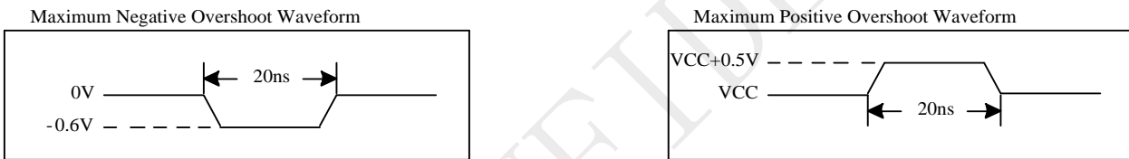
Figure 5-1 Maximum Overshoot Waveform
